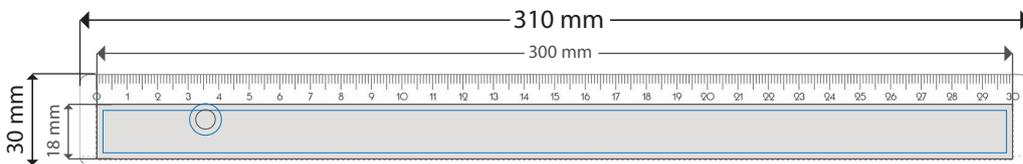
○ Ø 5 mm – POS Mitte 40 mm v. linker Kante, 15 mm v. unterer Kante
